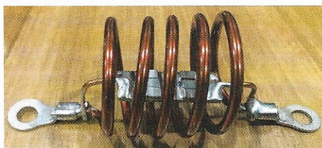
FIGURE 4: Construction of the 28.0MHz trap.
